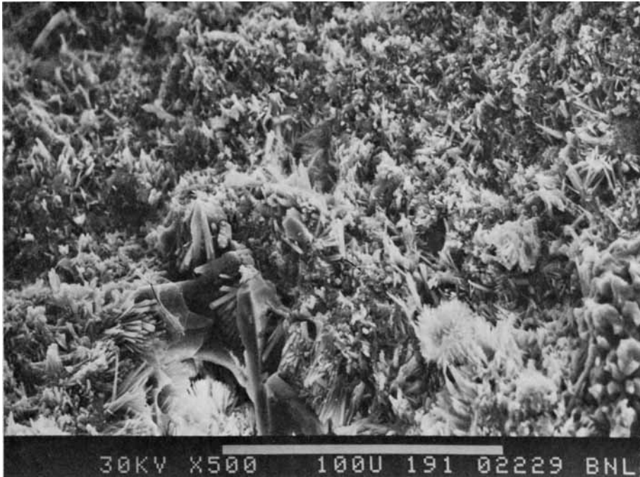
Fig. 7. Scanning electron micrograph of the fracture surface of hydrated C 3 S with a water to C 3 S ratio of 0.35 cured in an autoclave for 10 days.
