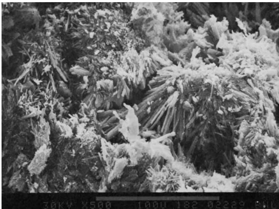
Fig. 8. Scanning electron micrograph of the fracture surface of C_3S -filled PMMA after exposure to brine.
